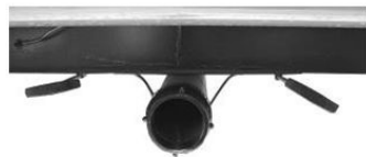
Black/Grey tank drain & valves
